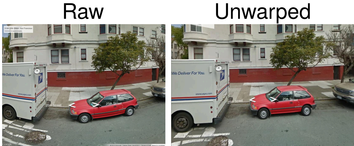
Figure 5.11: An example of the unwarping that needs to be done on images retrieved from Street View. Left: an image from Street View as initially scraped. The image appears warped ( e.g. straight lines in the real world are not straight in the image) due to the equirectangular projection used to store spherical panoramas. Right: the result of undoing this projection, which we do before using the images any further.
