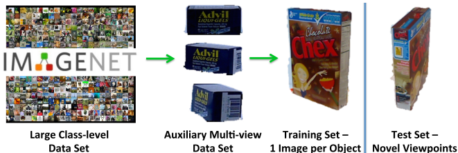
Fig. 1. Given only a single image of an object, we want to recognize this object from novel viewpoints. Traditional neural networks pre-train on ImageNet alone. We perform a multi-stage training procedure, in which we first pre-train on a large class-level dataset (left), followed by pre-training on an auxiliary multi-view dataset (middle), which trains our network to be robust to viewpoint changes. Finally, we train on the objects we wish to recognize from just a single image (right).
