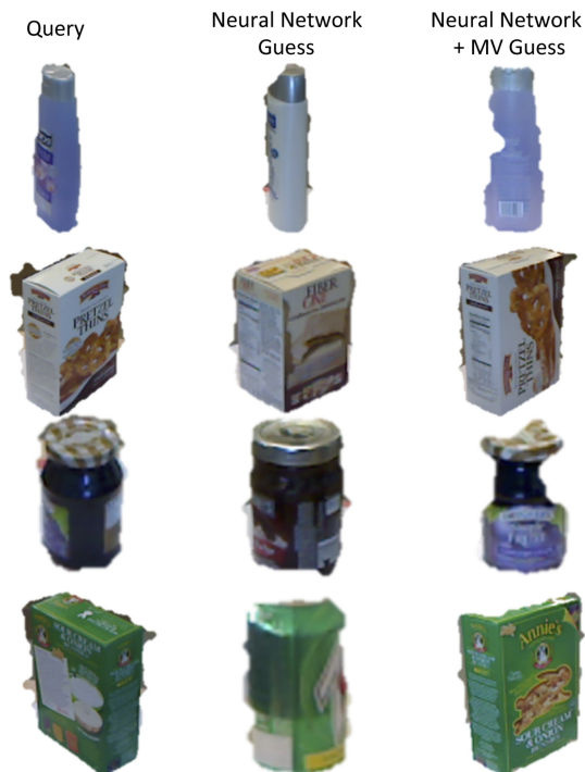
Fig. 4. Examples that were classified correctly using multi-view pre-training but were incorrectly classified using a neural network pre-trained only on ImageNet. Left: Query image. Middle: Guess by neural network pre-trained only on ImageNet (incorrect). Right: Guess with multi-view pre-training (correct).
